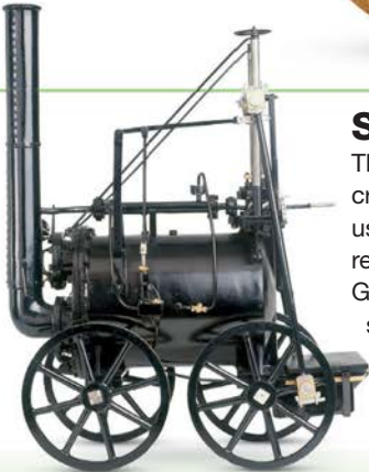
Model of early steam locomotive, built by Richard Trevithick c.1808
